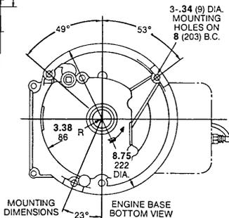
HOLE IN DECK FOR OIL SUMP TO BE 6.88 (175) DIAMETER. SUMP PROJECTION BELOW DECK MOUNTING FACE REQUIRES CLEAR SPACE. .56 (14) DEEP x 6.88 (175) DIA. PLUG CLEARANCE FOR OIL DRAIN PLUG.
