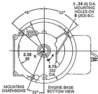
MOUNTING DIMENSIONS ENGINE BASE BOTTOM VIEW
